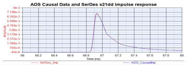
Notice that the two impulses are nearly identical. The ADS response no longer has the high frequency ringing on this peak.
