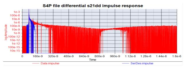
As can be seen, the SerDes impulse has less residual noise before the 67 nsec time delay and has no non-caual impulse re-growth at all.
