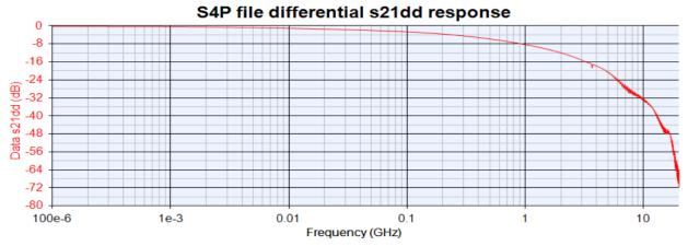
The frequency domain differential channel characteristics for this S4P files is shown here:
