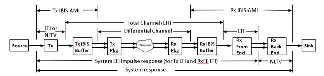
The differential channel often includes a transmit (Tx) package and a receive (Rx) package and is linear and time invariant (LTI).
